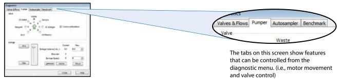
**Diagnostics Screen** - This screen demonstrates full control diagnostics, which allows for manipulation of all hardware components.
