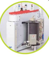
Wet Chemistry Panel – This panel holds the Inorganic Carbon (IC)
