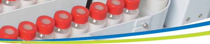
Sample Conveyor – The Lotix conveyor systematically moves sample vials to and from the sample position for sample introduction via the needle assembly. The conveyor is designed to hold 30 – 40 mL VOA vials.
