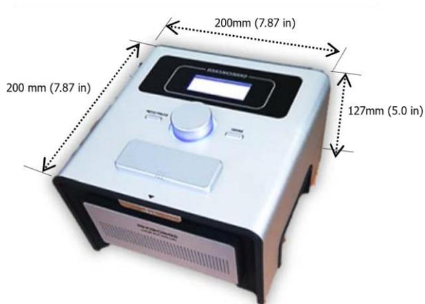
**Figure 2** Dimension of instrument with the drawer opened
