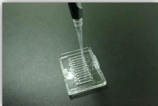
After preparing the reaction sample, aspirate with a pipette and vertically place the tip in the inlet hole like shown in Figure 18. The inlet hole is next to the printed well number and size of this hole is a bit bigger than outlet hole (Refer to Figure 13). The hole on the opposite side of the well is outlet whole where the air existing in the well and excess volume of the sample is going out.
