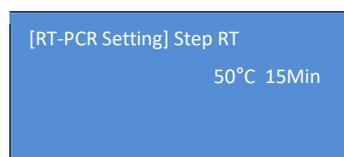
The screen on the left is displayed when you select "Set Protocol" from the menu screen. This screen is for setting RT (Reverse Transcriptase) PCR cycle. If you press jog dial, the number 50 in left screen starts to blink.
