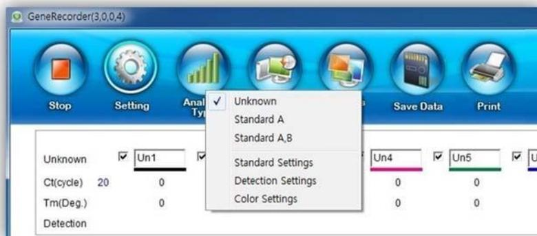
The user can choose type of analysis using "Analysis Type" menu. By clicking the button the user can choose one from following three analysis types. Default type of analysis is "Unknown".
