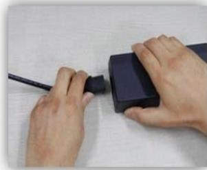
**Figure 11** Connecting DC adaptor and USB cable to the instrument
