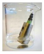
Figure 35. Nebulizer Cleaning (not more than 2 cm of cleaning liquid)
