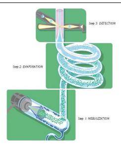
Figure 2. Cross-sectional View of the Detector
