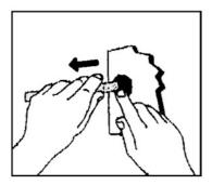
To remove the tube, disengage the grab ring teeth by a simple manual pressure on the push sleeve and withdraw the tube from the fitting.
