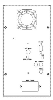
Figure 6. Rear Panel of the detector
