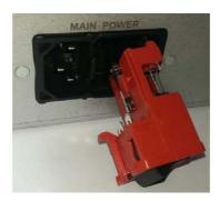
Figure 36. Power socket fuse chamber with spare fuse shown (on the left)
