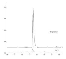
Figure 27. Chromatograms of Caffeine with ELS detection at various evaporation temperatures
