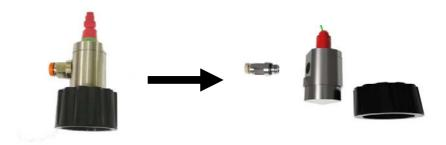
Figure 34. Nebulizer preparation for cleaning
