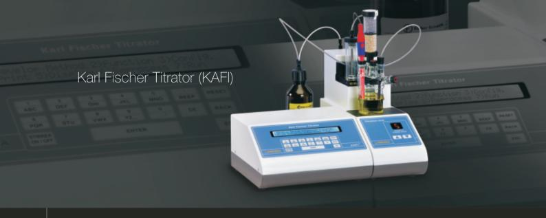
Karl Fischer titration is an accurate, rapid and efficient method for determining the water content in samples. When the sample is titrated in the presence of  $SO_2$ ,  $I_2$ , and an organic base, moisture from the sample extracted in the solvent, can be quantitatively estimated. Dry methanol is used as a solvent in Karl Fischer titration.
