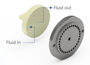
The flow path in the valve rotor is specifically designed with a hidden channel so that the sample liquid has minimum contact with the stator surface when the valve is turning. This feature is very effective in avoiding contamination of sticky compounds (such as benzopyrene) on the stator surface.
