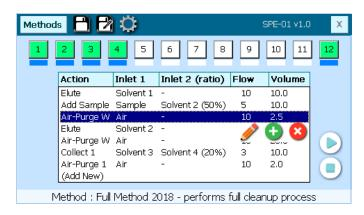
The SPE-01 now comes equipped with a resistive touch screen interface that works even under wet conditions. Sample selection and method editing can be intuitively performed in just a few steps. When running, the screen highlights the current step being run and displays its processed volume.
