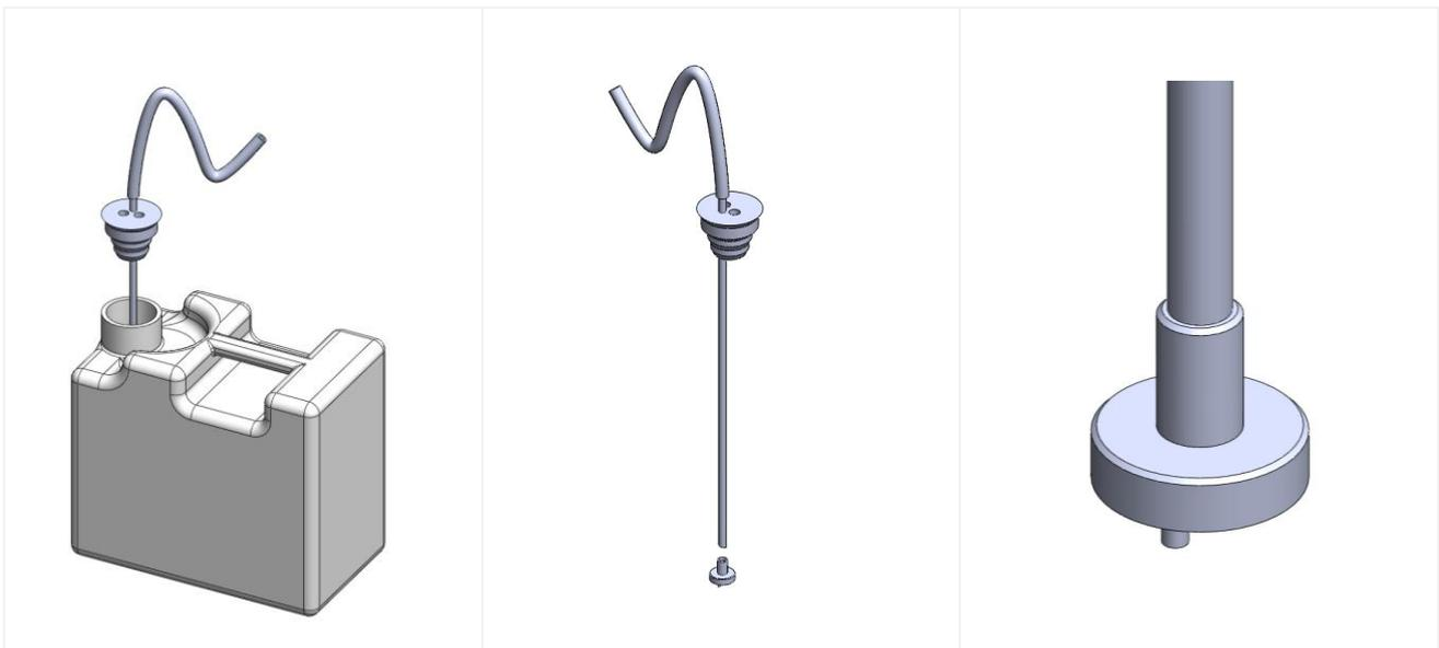
*fig. 34 – Detergent intake **STANDARD** version. Fitting the detergent intake pipe to the can. Fit the rubber cap over the top of the can for a perfect, secure connection. The pipe is supplied complete with intake filter.*
