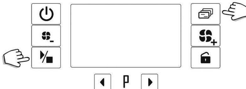
fig. 39 – RESET cycle selection buttons ("Start/Stop" + "Functions") buttons
