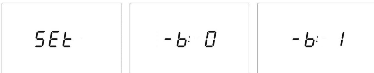
fig. 30 – **SET** appliance parameters; parameter **-b** is used to enable and disable overwriting of the internal data memory.
