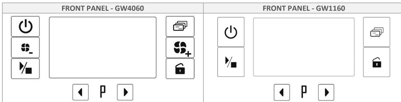
fig. 4 – Front panel; the central part contains the segment display and the appliance control buttons.
