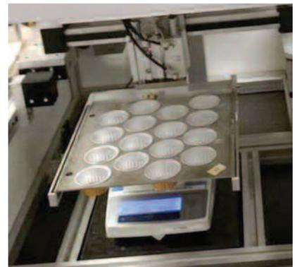
Weighing of samples before drying to assess dryness or after ashing can be done with SEAL robotic systems or inline with various other steps on our MiniLab robotic system.
