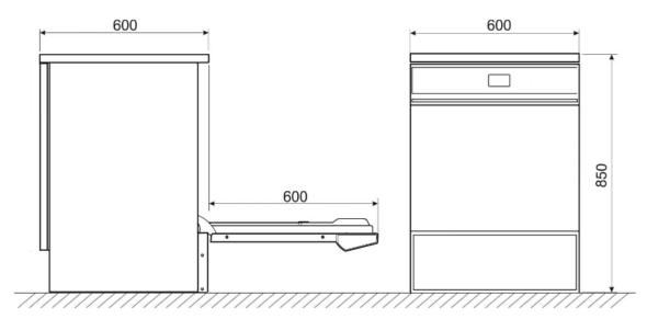
■ H=830 mm for built-in mounting solution by removing top and H=1250 mm by installing a frame or a plinth
