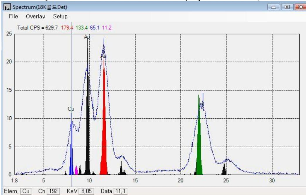
The overlapped spectrum is acquired by proportional counter and main spectrum is acquired by Si PIN detector for 18K Gold alloy. These spectra show the different resolution for the same sample since resolution of counter is around 1,200eV and PIN detector is 149eV. If the peak is not identified automatically move cursor to center of the spectrum then the bottom of the
