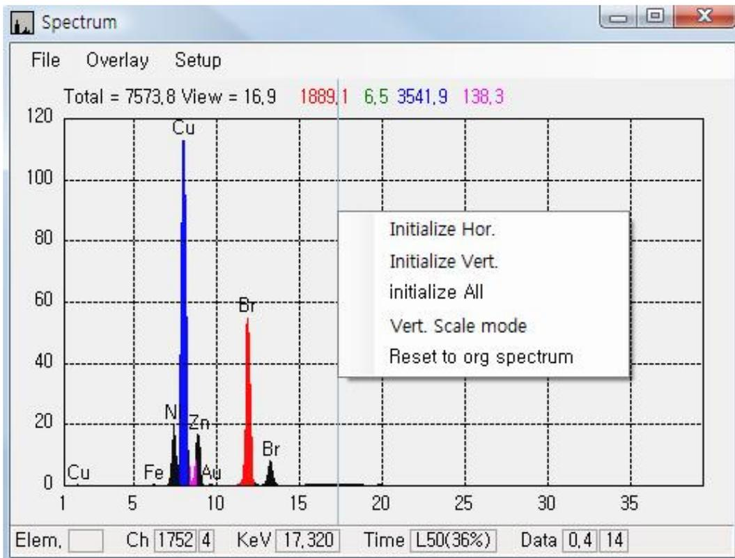
Click Right button shows menus to initialize, expand/reduce the vertical scale and reset to original spectrum.
