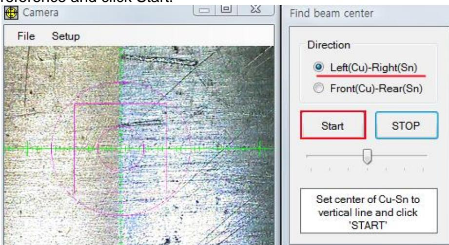
When system finish to find the center of beam, make sure the vertical line coincide with border line between Cu and Sn. If does not, Go setup -> Adjust scale position.
