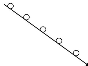
$$\text{Moving distance} = (\text{Start} - \text{Stop}) / (\text{Meas. point} - 1)$$
