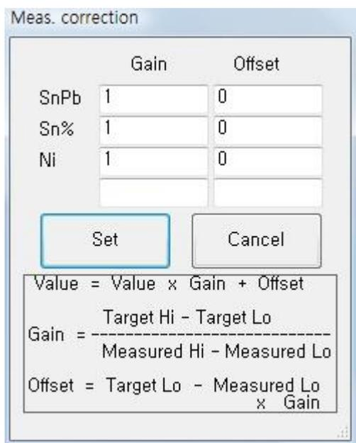
Gain=1 Offset=0 is default value which means measuring correction is not effected to result.
