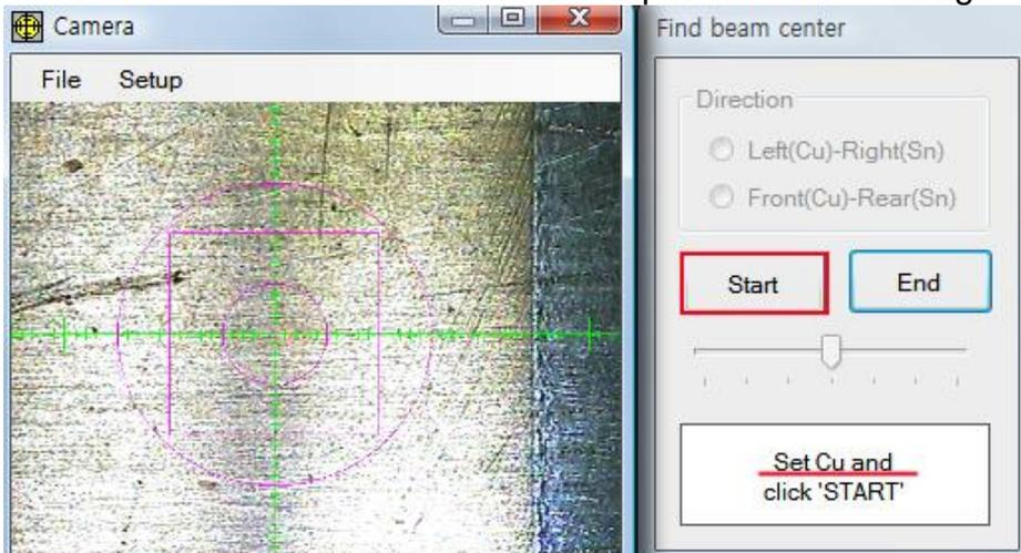
Place center of camera to border line between Cu and Sn of the position reference and click Start.
