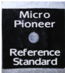
System Adjust is for positioning to the right energy location of the known peaks in KeV using Reference Standard which is contained Cu and Sn.
