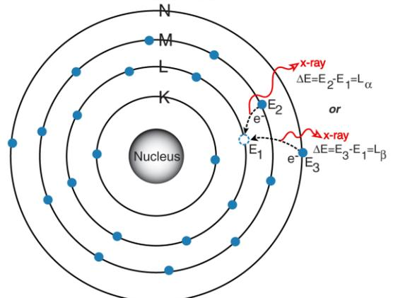
3) When a vacancy is created in the L shell by either the primary excitation x-ray or by the previous event, an electron from the M or N shell “jumps in” to occupy the vacancy. In this process, it emits a characteristic x-ray unique to this element and in turn, produces a vacancy in the M or N shell.
