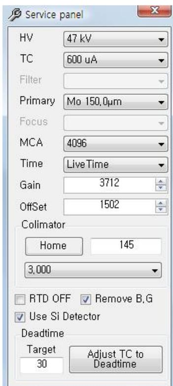
Place cursor on Main window and click the Main window then press Alt+Ctrl+Shif simultaneously and hold these keys and type "pioneer" and Press Enter key. Then service menu will appear in spectrum window. Click Service menu on the Spectrum window.
