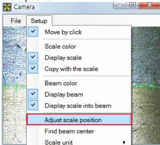
Adjust vertical line to border line between Cu and Sn. Click SET.
