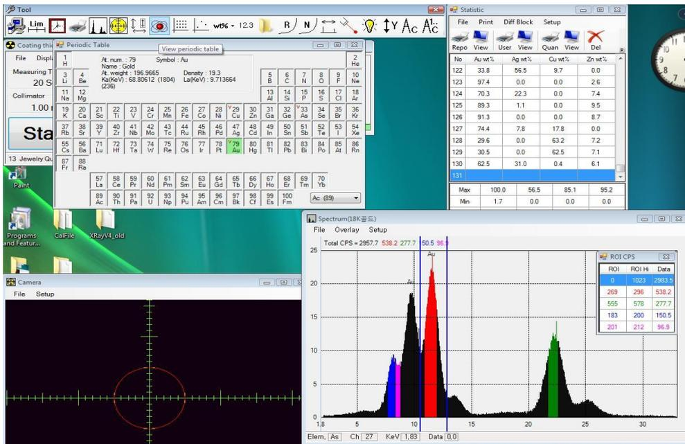
Clicking specific element shows its information such as Atomic number, Energy Value etc. and two vertical lines (blue lines) which is ROI low and ROI High are placed on the Spectrum window. Below is example of clicking Au.
