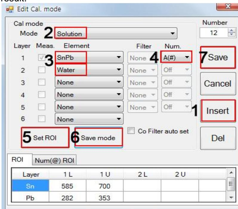
Select Cal. Mode which is just created. Select biggest collimator and set measuring time as 100 sec. High Voltage must be adjusted regarding measuring element.
