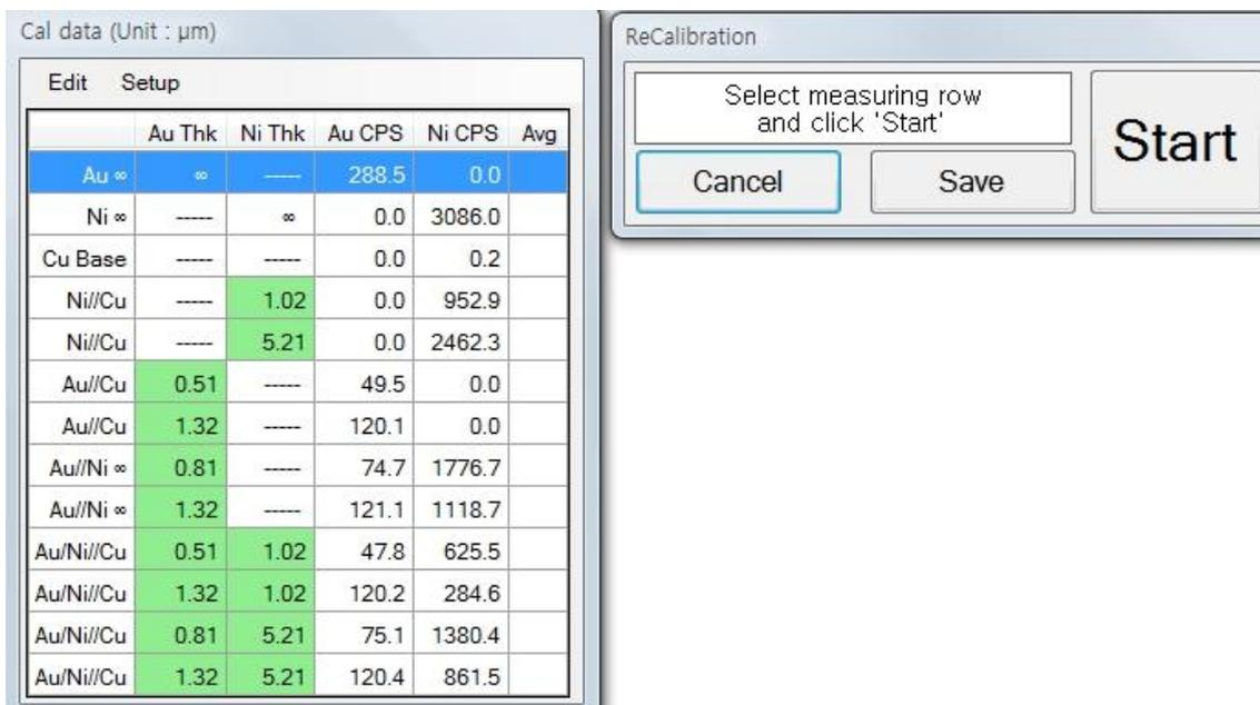
The screenshot shows two windows from the XRF-2000 software. The 'Cal data (Unit :  $\mu\text{m}$ )' window displays a table of calibration data. The 'ReCalibration' dialog box is overlaid on top, prompting the user to select a measuring row and click 'Start'.
