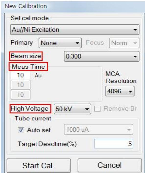
Double Click on Beam size, Meas Time and High Voltage, then Edit Cal. Mode window appears. Do as shown below. Try to change numerical filter to get better result.
