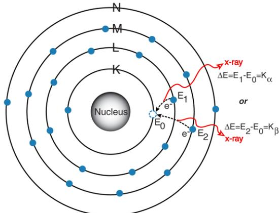
2) An electron from the L or M shell “jumps in” to fill the vacancy. In the process, it emits a characteristic x-ray unique to this element and in turn, produces a vacancy in the L or M shell.
