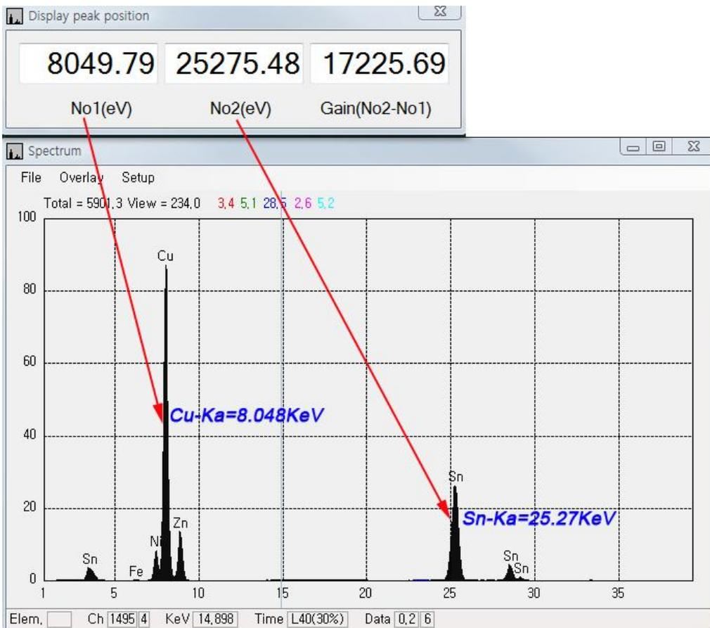
To display Peak Information, place cursor on the Spectrum Screen then press Alt+P simultaneously.
