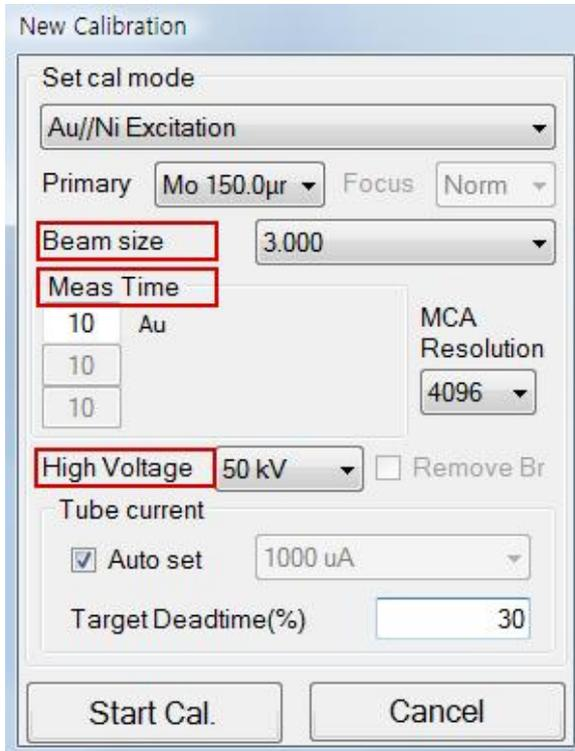
Double Click on Beam size, Meas Time and High Voltage, then Edit Cal. Mode window appears. Do as shown below.
