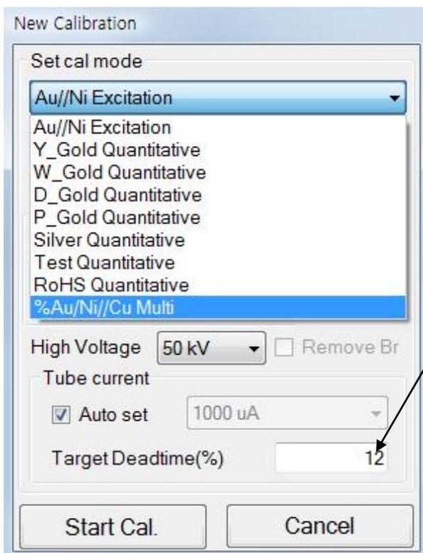
Target Dead time is 5% for Proportional Counter, 30% for PIN Diode detector.
