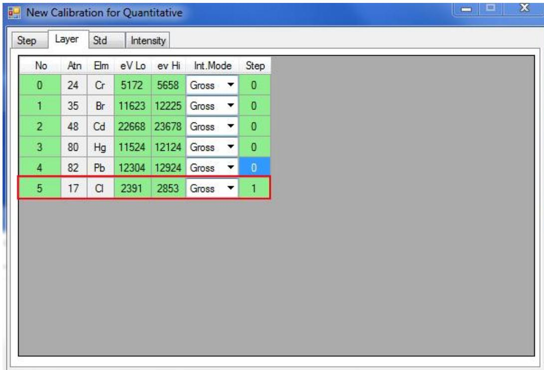
The screenshot shows a software window titled "New Calibration for Quantitative". It contains a table with columns for Step, Layer, Std, and Intensity. The table lists six calibration steps for various elements. The last row, representing Chlorine (Cl), is highlighted with a red border, indicating it is the current layer being configured.
