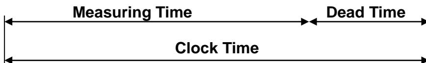
The Clock Time is corrected for the Dead Time, always meaning:
