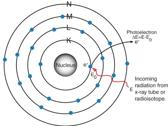
1) An electron in the K shell is ejected from the atom by an external primary excitation x-ray, creating a vacancy.
