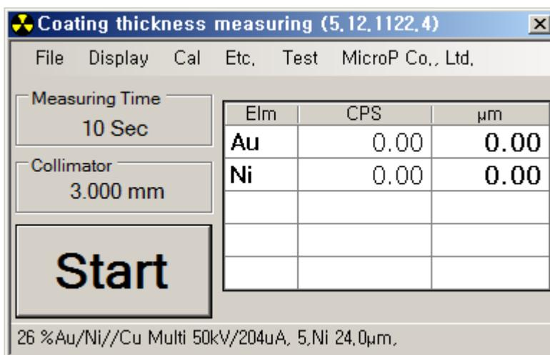
Indicate Measuring Time, Collimator Size, Start and Stop Button, CPS Information, Result of Thickness or Concentration and Measuring Mode. Start Button toggles start and stop to measure.
