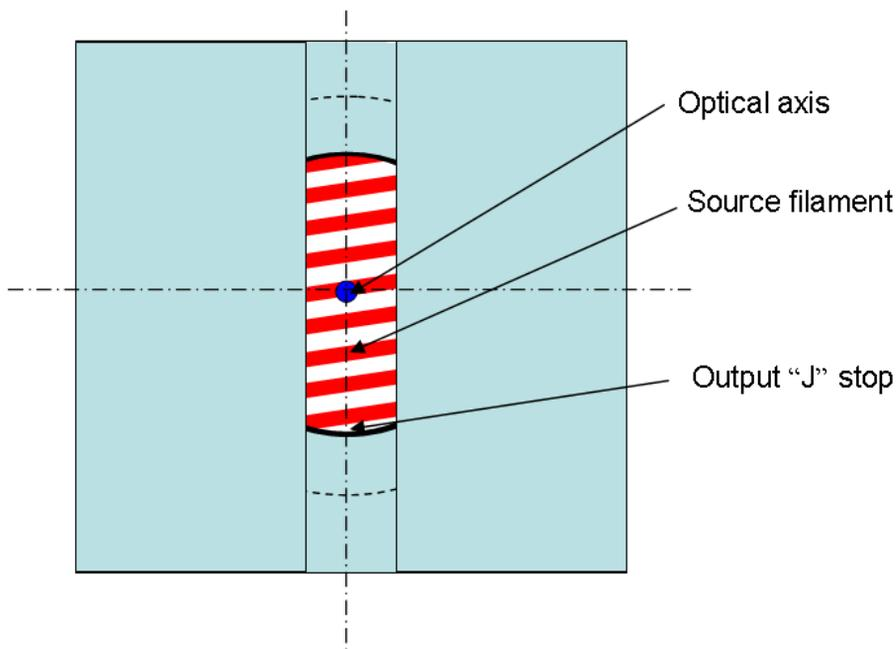
Figure E- 3. Illumination distribution with vial sampling accessory
