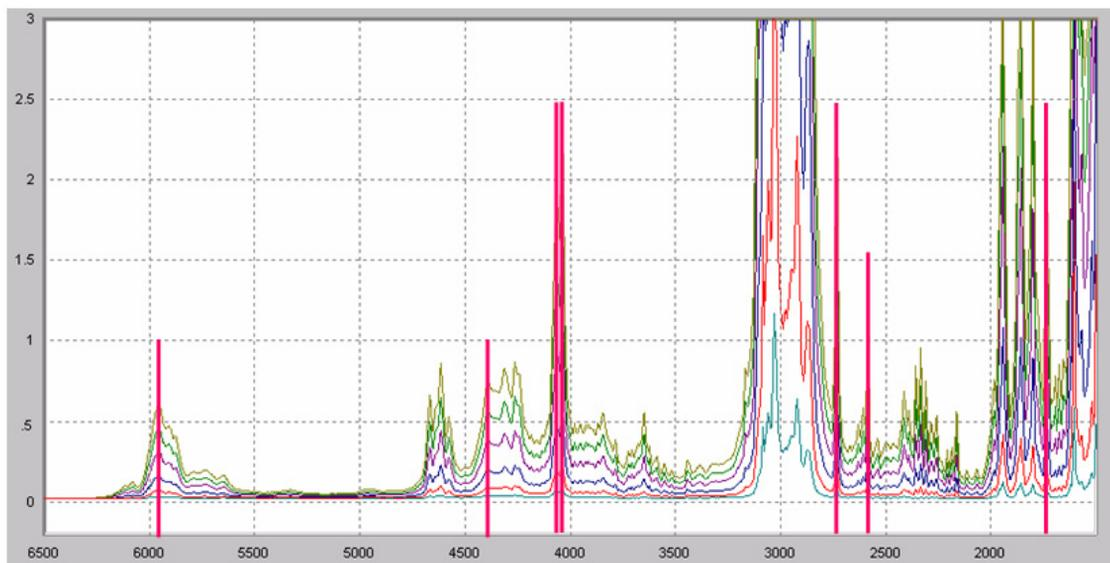
Figure C- 1. Series of toluene spectra
