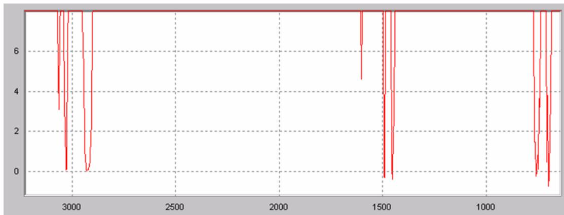
Figure C- 4. Expanded view of figure 3 showing transmittance near zero%. The deviation from zero transmittance for the 6 bands is  $\pm 0.1\%T$
