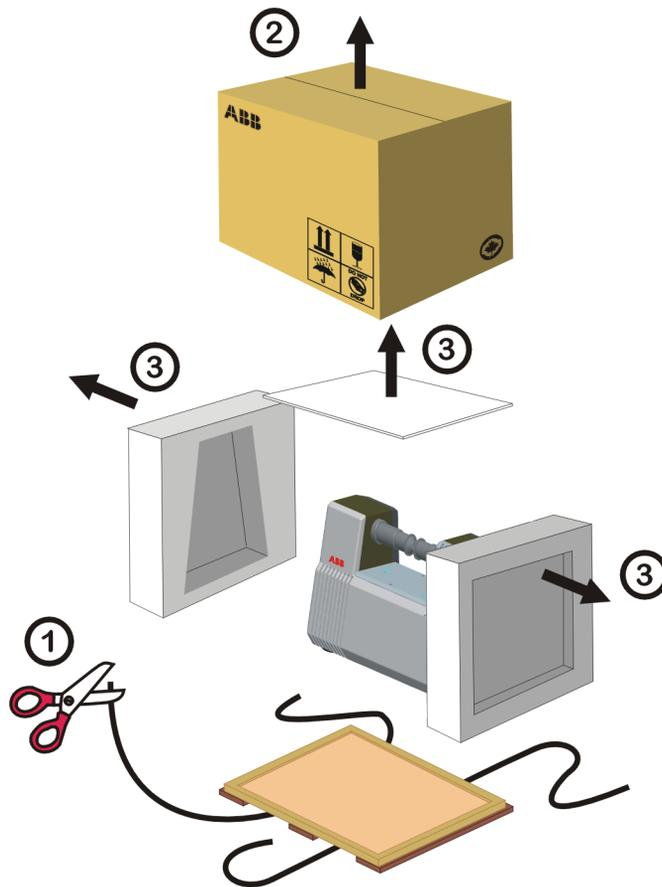
Figure 3- 1. Unpacking the spectrometer
