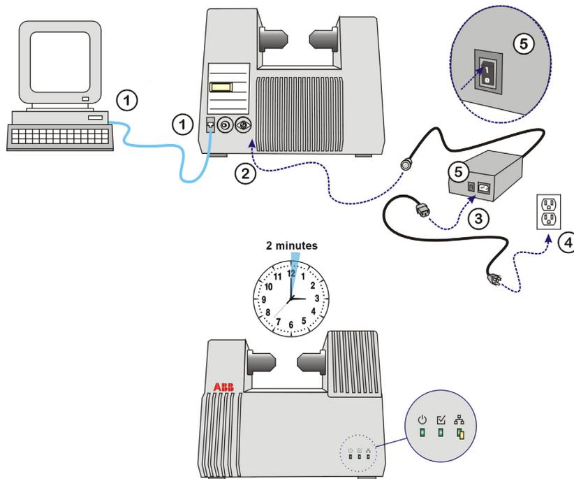
Figure 3- 2. Installation procedure: direct connection
