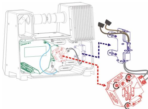
Figure 7- 4. Source module: Source control board and source
