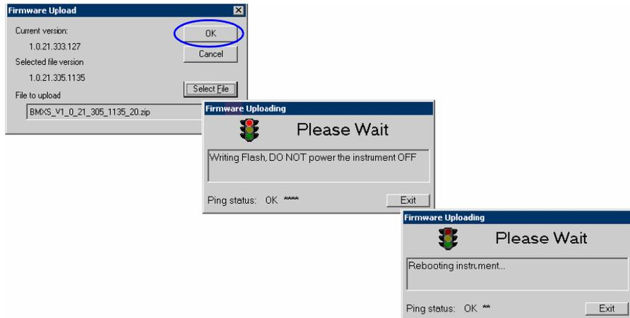
Figure B- 4. Uploading firmware
