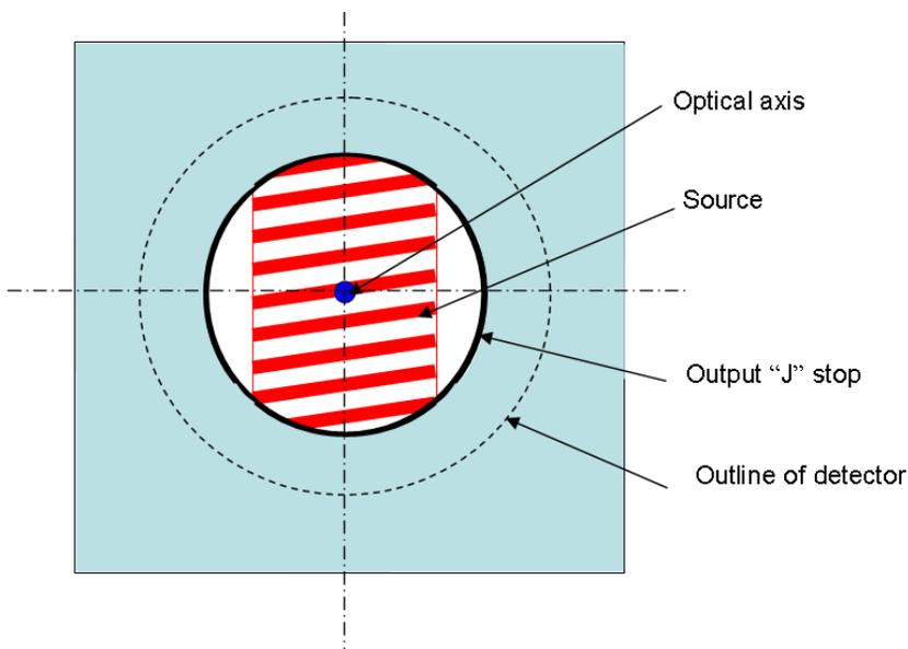
*Figure E- 1. different field of view defining elements for the MB3600 with Quartz halogen source*
