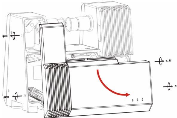
Figure 7- 3. Front panel captive screws
