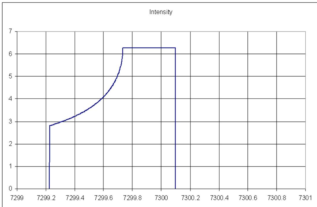
Figure E- 2. Illumination distribution as a function of frequency shift for figure 1 distribution
