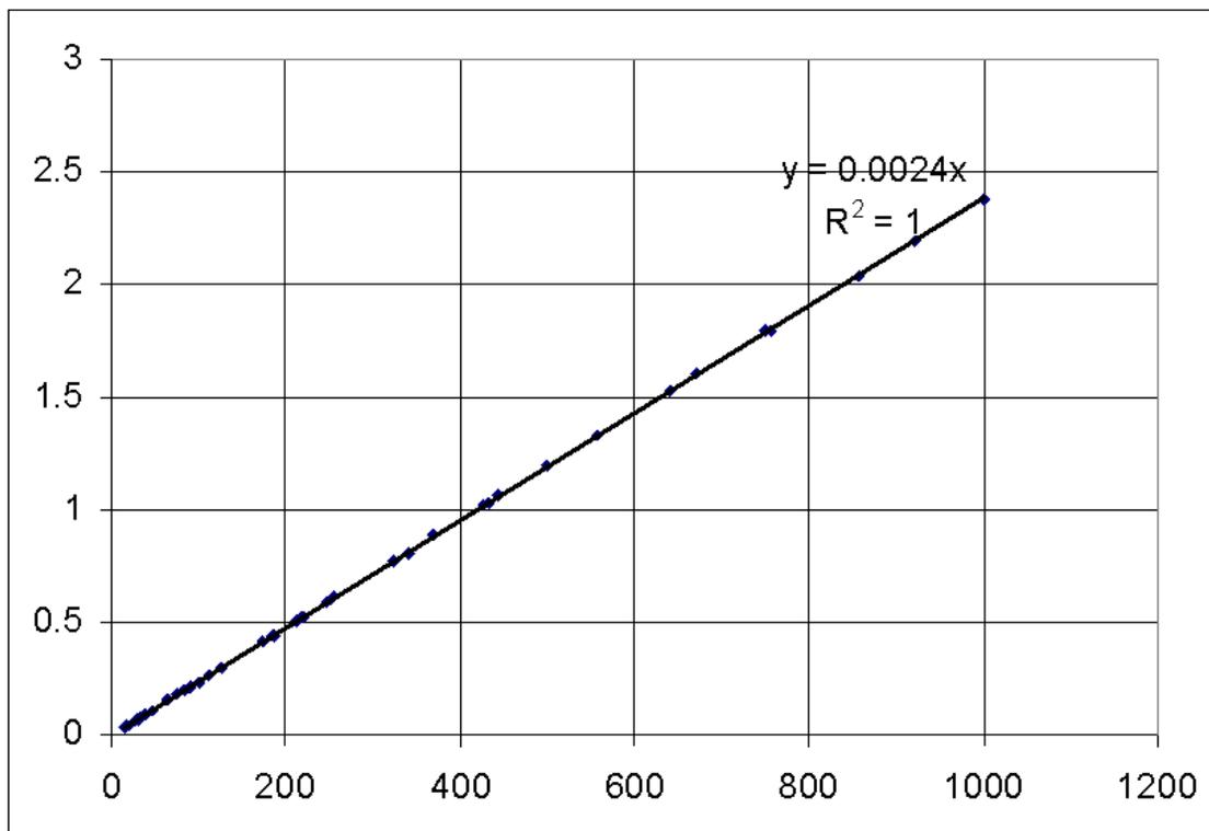
Figure C- 2. Absorbance vs normalized pathlength for 6 absorbance spectra at 7 frequencies
