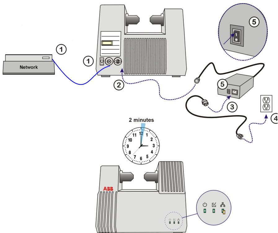
Figure 3- 3. Installation procedure: Network connection
