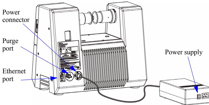
Figure 6- 1 : Connector location
