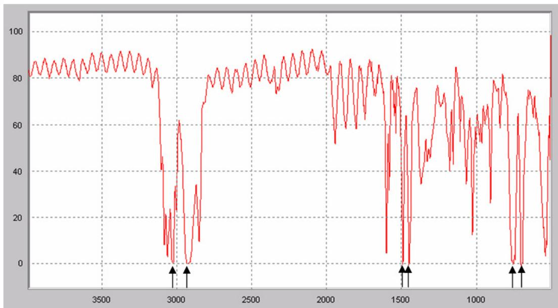
Figure C- 3. Transmittance spectrum of polystyrene film indicating the 6 total absorbing bands
