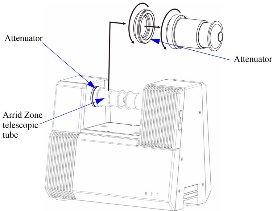
Figure 6- 2. Attenuator location
