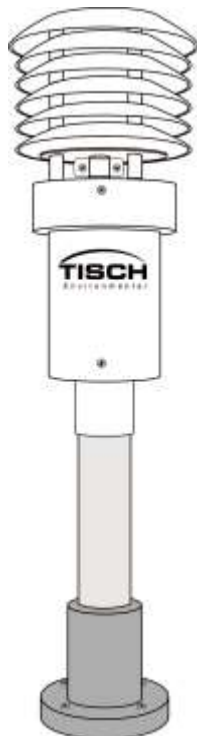
Picture showing the TE-FRM-CAL calibration head inserted onto downtube
