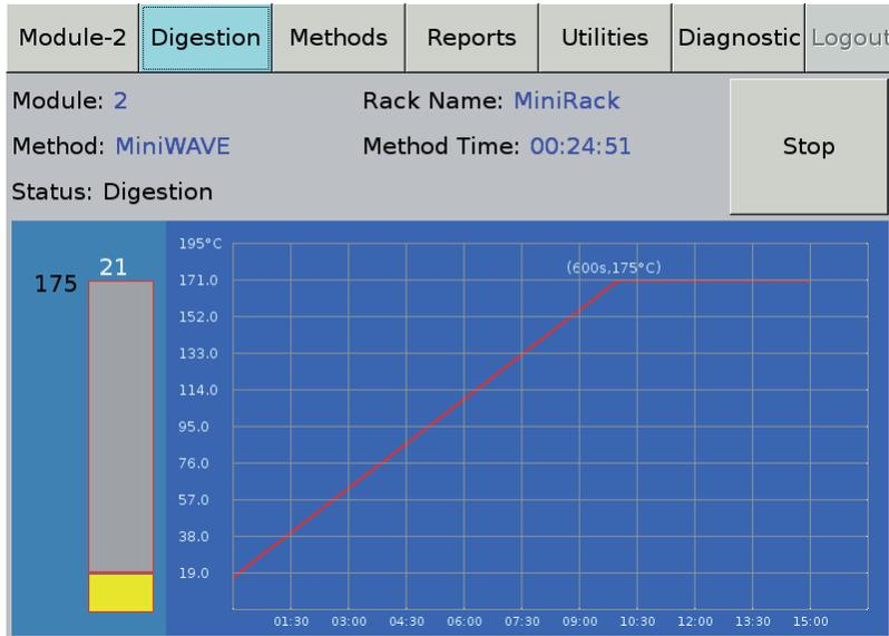
During the digestion this screen informs the operator of the progress of the digestion.
