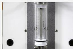
Precision Syringe for 5 and 25 mL Samples with Automated Sample Dilution
