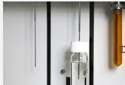
Separate Water and Soil Needles to Prevent Cross-Contamination
