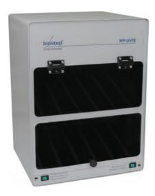
The HP-UVIS combines two UV-tubes for 254/366 nm in one unit.
