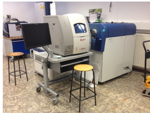
CESI8000 coupled to 5600 TripleTOF MS
