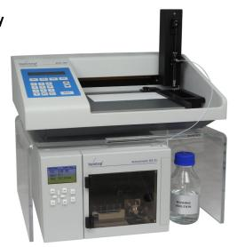
The association of the BS35 auto-sampler with the AS30 HPTLC applicator offers a set of fully automated sample depositions on TLC plates.
