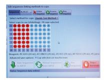
**6. Sequences Screen** – This screen will be the day-to-day operations screen. To set a sequence, you choose a method, choose which cups you wish to use, and give the sequence a name. If using the PC to control the unit, you can start the sequence by clicking the "Run Sequence Button". If the touch-screen controller will be used to run the sequences, you must click "Save Sequences to ABFill" in order to have them available.
