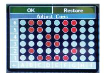
Adjusting the selected cups is done in a similar manner to using the PC software; individually, in rows, in columns, or the entire block. Press "OK" after the correct cups have been assigned.
