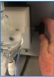
**16.3** Once lowered, thread the drying cartridge into place by twisting it counterclockwise onto the nut at the exit port of the extraction head.
