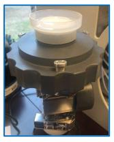
**13.13** Lift the entire assembly onto the top of the unit and line up the pin inserts into the slots on top of the unit.
