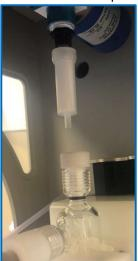
**16.4** Lift the glass chamber assembly up and ensure the tip of the drying cartridge slips into place in the nut at the sample entry port of the glass chamber.
