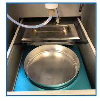
17.4 Close the cover to ensure the hexane fumes are directed out of the unit via the exhaust system. Failure to do so can cause harm to the analyst if hexane fumes are inhaled. Failure to close the cover will prevent hexane from getting into the aluminum pan and cause sample loss.
