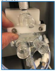
**7.3** Using a 5/32 hex nut driver, tighten the 2 screws to secure the glass chamber in place.
