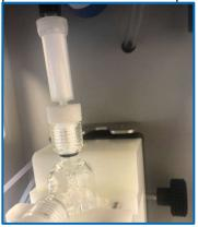
**16.5** Tighten the wheel screw to lock the glass chamber assembly into place.
