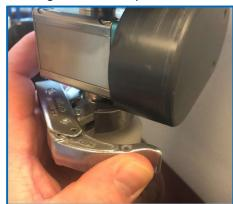
**13.12** Place an SPE disk assembly onto the extraction head (47mm or 90mm) and twist to tighten.
