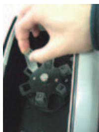
Specify measurement parameters, and then load a sample to each cell
